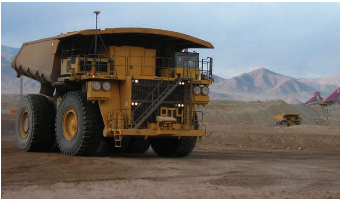
Komatsu's autonomous trucks have no driver and follow a determined route based on GPS technology
