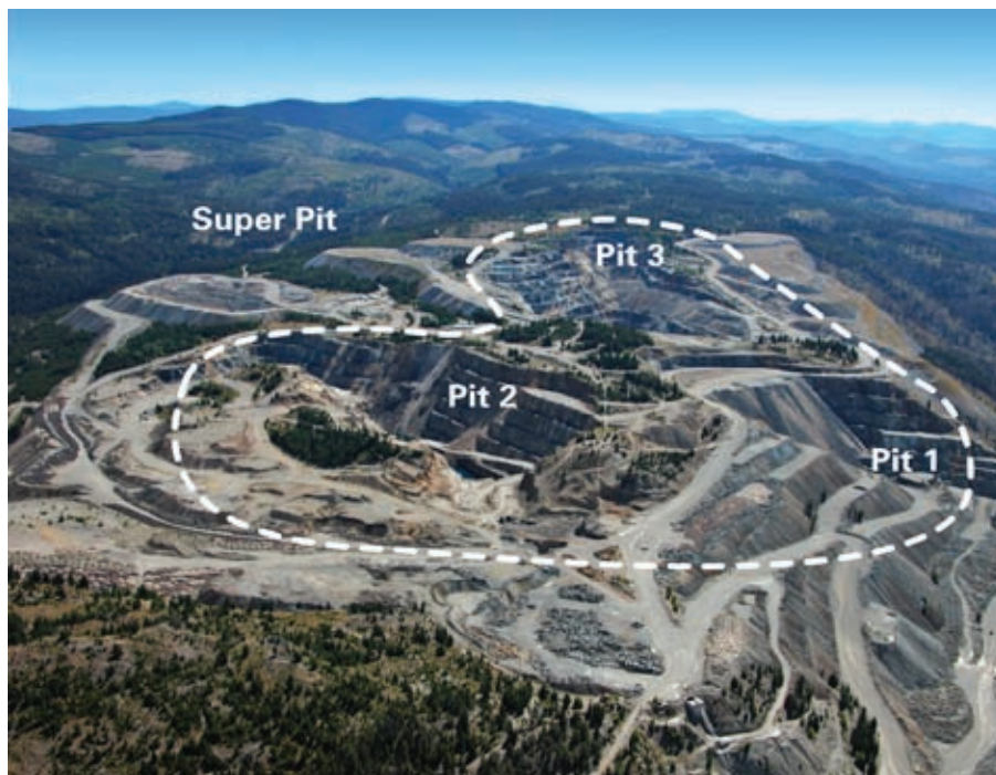
These are the three developed pits that will form the Super Pit
